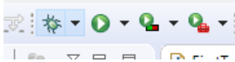
Picture 10: Executing the application in debug mode by pressing the green bug
